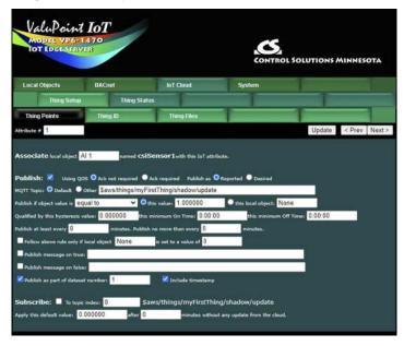
The MQTT publish and subscribe "rules" are created with an easy to use template. A diagnostic page is also provided where you may view the most recently published data, and publish arbitrary JSON formatted data for testing purposes. The entire configuration is saved in the internal Flash file system in XML format. This file may be exported to replicate additional copies of the configured device, or for backup.
