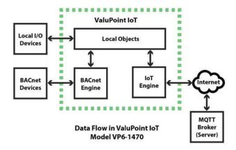
The VP6-1470 also supports interactive dashboards using ThingsBoard. The VP6-1470 includes features specific to ThingsBoard that allow MQTT interaction with graphic widgets on the dashboard. BACnet data published by the VP6-1470 can show up as real-time gauge indications or charts. Input from the dashboard such as knob adjustments or switch changes will be immediately reported to the VP6-1470 and those changes are immediately accessible as BACnet data.
