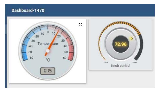
Our csiActuator3 is mapped to the Analog Valus 6 object for our demo. When you move the knob on the web page in Thingsboard, the AV 6 value will change accordingly.
