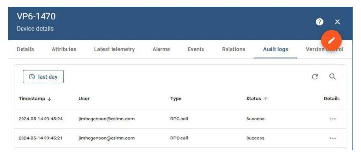
The Audit logs show all RPC calls that were involved in making any control widgets work. Click on the Details icon to see the entire exchange between Thingsboard and our MQTT device.
