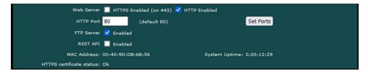
Secure browsing can be enabled here, and non-secure can be disabled. You cannot disable both, and a forced configuration reset will restore HTTP (non-secure) web browsing. In order to use HTTPS, you must first upload the necessary SSL certificates (see Appendix G) or allow the certificates to be self-generated by explicitly deleting existing certificates.
