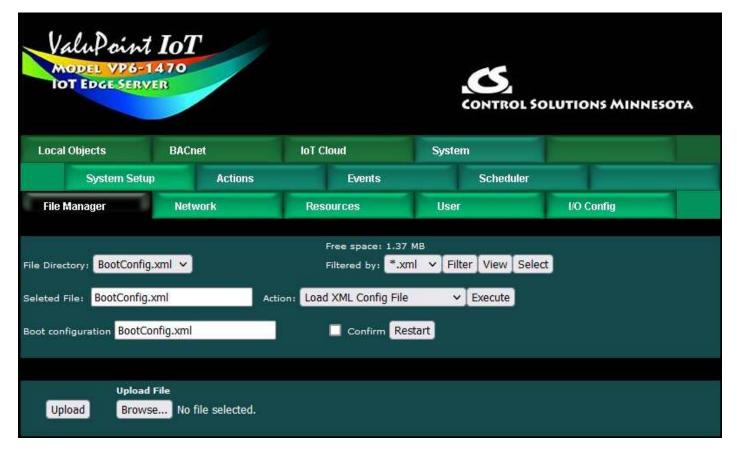
The File Directory is a list of files that are currently stored in the ValuPoint's Flash file system. To filter files by type, select a type from the Filtered by list, and click Filter.
