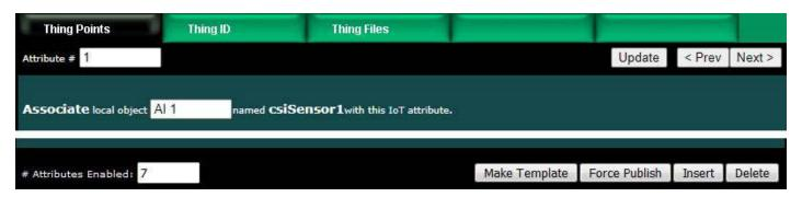
Insert will insert a new attribute before the attribute number shown, and is used for placing attributes between existing attributes. It is not necessary to use Insert to add attributes to the bottom of the list or to redefine any attribute presently having zero for an "associate" object. Attribute numbers work like row numbers in a spread sheet.
