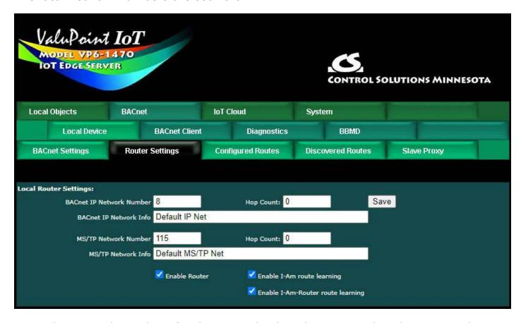
Enter the network numbers for the networks directly connected to this router. These must be unique across the entire internetwork. These numbers will ultimately tell other routers how to find devices on these local networks.
