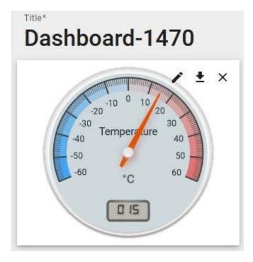
Our point csiSensor1 is being displayed on the gauge, and it is getting its data from a remote Modbus device.
