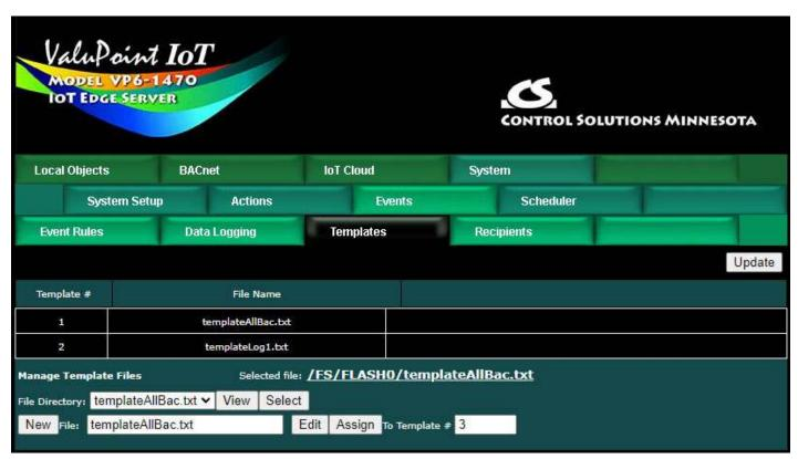
The template is a simple text file with a .txt suffix and could be edited externally and uploaded via the File Manager page. It can also be edited here.
