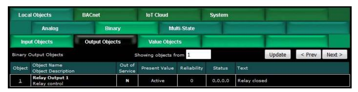
The object name, value, and status are shown for a list of objects starting with the number entered at the top of the page. Click Prev/Next to scroll through the list. Click on the object number in the first column to change name or out-of-service state.
