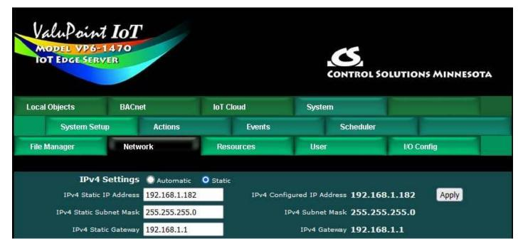
Select either Static or Automatic for IPv4. To change the Static IP address of this device, enter the address, subnet mask, and gateway, then click Apply. Select Automatic to specify that DHCP should be used to obtain an IP address upon power-up. IP address change will take effect upon next power cycle.
