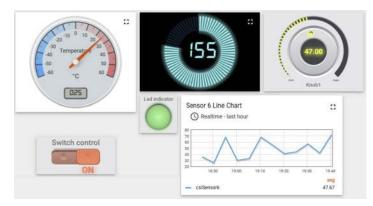
The VP6-1460 also supports interactive dashboards using ThingsBoard. The VP6-1460 includes features specific to ThingsBoard that allow MQTT interaction with graphic widgets on the dashboard. Data published by the VP6-1460 can show up as real-time gauge indications or charts. Input from the dashboard such as knob adjustments or switch changes will be immediately reported to the VP6-1460 and those changes are immediately accessible as Modbus data.
