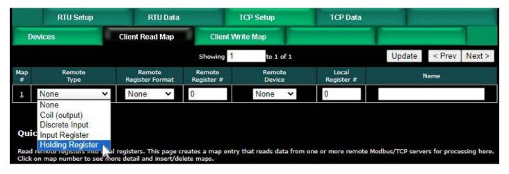
To create a Read Map, start by selecting the Modbus register type to read from the drop-down list.
