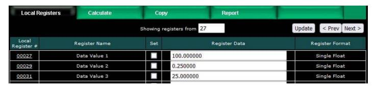
Constants may be introduced into the calculation by reserving a register to hold that constant, and then configuring it to apply a default value at power-up. This default
