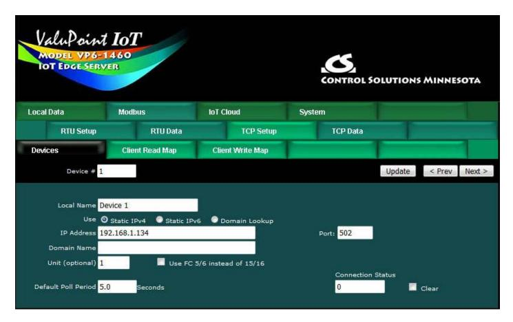
A unit number is always included in each Modbus TCP packet. This is the equivalent of the RTU slave address. Some TCP devices pay no attention to unit and simply echo back whatever you had sent. However, if you are accessing RTU devices on the other side of a TCP to RTU router (gateway), then the unit does become the RTU slave address on the RTU side of the gateway and multiple RTU devices are accessed at the same TCP IP address.
