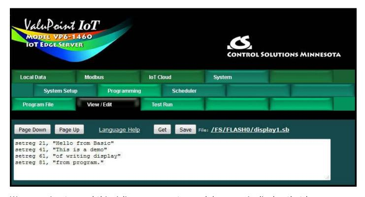
We are going to send this 4-line message to an alphanumeric display that has a Modbus RTU interface. To start out, we need to configure the Modus RTU port for the baud rate that matches the display. The ValuPoint will be the master since the display is an RTU slave.
