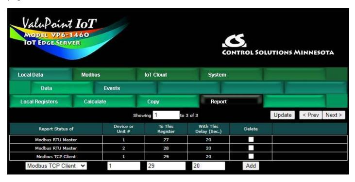
This optional list allows reporting device errors as register values to make it easier to monitor communication failures. The length of the list is variable. To add to the list, select the type of device to report on, select the device instance or unit number to report on, and select a register in which to put the status indication. Enter a delay if desired, and then click Add.
