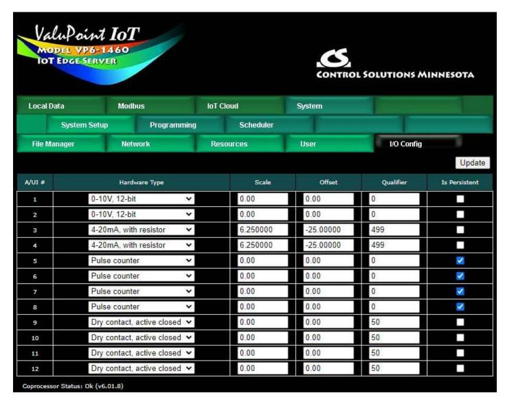
The relay outputs do not require any configuration. The analog/universal inputs do require configuration on the I/O Config page. Select the desired input type and enter additional parameters as applicable.
