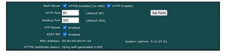
Secure browsing can be enabled here, and non-secure can be disabled. You cannot disable both, and a forced configuration reset will restore HTTP (non-secure) web browsing. In order to use HTTPS, you must first upload the necessary SSL certificates (see Appendix D) or allow the certificates to be self-generated by explicitly deleting existing certificates.
