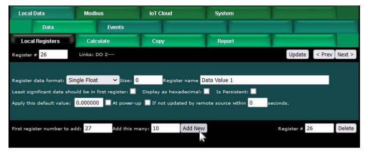
We have now created 10 new floating point registers. The important thing to observe here is the register numbers in the first column. Remember that Modbus protocol assigns register numbers (or addresses) in 16-bit increments. Since single precision floating point registers are 32-bit registers, each floating point value occupies 2 spots in the Modbus register map. The local register number assignments reflect this fact.
