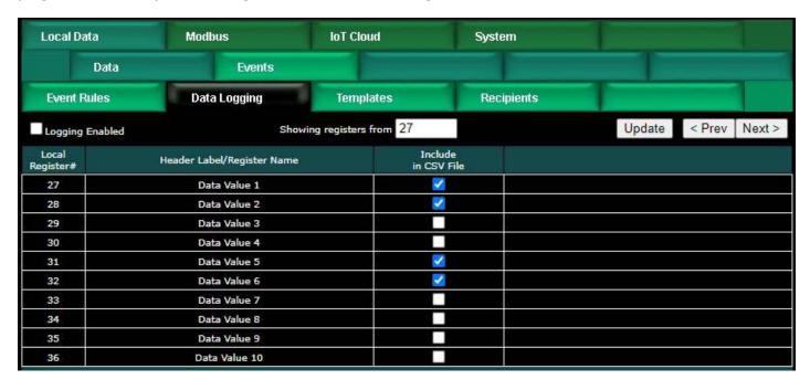
Note the Logging Enabled check box in the upper left corner. You must disable logging while making changes to logging parameters or register selections. Then check the Logging Enabled box and click Update to enable logging. The Logging Enabled state is retained through power outages, and logging will resume when power is restored if it was enabled to begin with.
