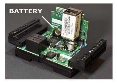
Replace battery with BR1225A only. Use of another battery may present a risk of fire or explosion. Replace with battery polarity as marked on the circuit board. Reverse polarity of the battery will not damage the board, but the clock will not be backed up if the battery is reversed.
