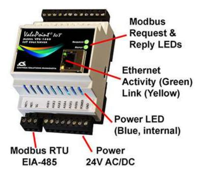
VP6-1460 Request and Reply LEDs reflect Modbus RTU traffic, and the Ethernet activity LED will indicate network traffic in general. If Modbus RTU is not being used at all, then the Request and Reply LEDs will indicate TCP traffic. If Modbus RTU is in use, then the Request and Reply LEDs will indicate Modbus RTU traffic while the Ethernet LEDs will be the only indication of TCP traffic.
