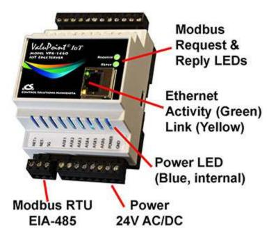
(b) Connect a CAT5 cable between the RJ-45 jack on the ValuPoint, and your network switch or hub. You cannot connect directly to your PC unless you use a "crossover" cable.
