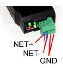
DO NOT connect power to the terminal block on the adapter. The adapter gets its power from the USB port of your PC. The adapter only draws a very small amount of power, well below the limit provided by standard USB ports.
