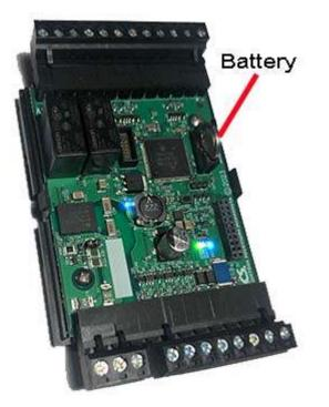
Replace battery with BR1225A only. Use of another battery may present a risk of fire or explosion. Replace with battery polarity as marked on the circuit board. Reverse polarity of the battery will not damage the board, but the clock will not be backed up if the battery is reversed.
