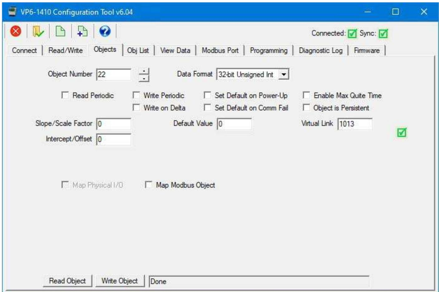
Example of usage: If you want to read via Modbus how much time the relay output DO 1 on the VP6-1410 (object 13) has been in the on state, you would enter virtual link number 3013 in some otherwise unused object. Now read this object via Modbus to see how much time DO 1 has been in the on state.
