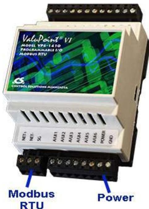
Connect power to the terminals marked POWER and GND. Connect the RS485 network to NET+, NET-, and SG. The serial communication signal ground marked SG is NOT electrically common to any other GND terminal on the device, and therefore must be connected to the network signal ground in order to complete the communication connection.
