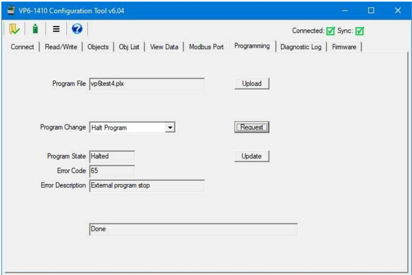
If the program encounters a fatal error during execution, its error code and description will be displayed after clicking the Update button. The Update button causes the tool to query the ValuPoint device for status.
