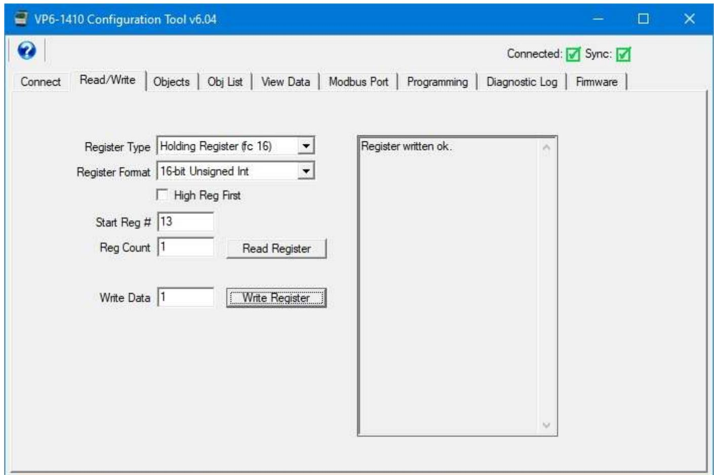
Select all of the same parameters that you would for reading a register. In addition, enter a data value to be written, and then click 'Write Register'. The 'Register Format' will be used to determine how the data you enter is converted to raw binary form to be transmitted to the device. The result of your 'Write Register' attempt will be displayed in the log window. The example illustrated above will turn on relay DO 1 in the VP6-1410.
