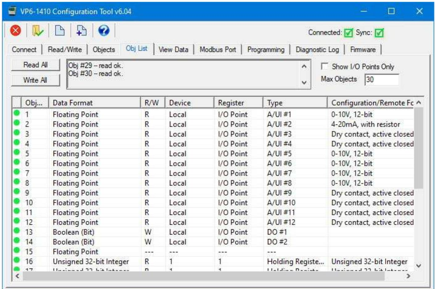
Click 'Read All' to begin the process of reading all of the available object maps from the device. If the tool was not in sync with the device previously, the red dots in the first column will turn green as the map on that line is updated and synced with the device.
