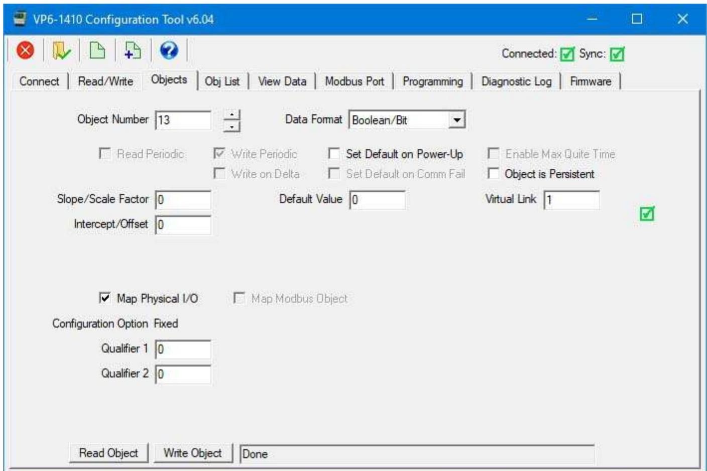
There are many other possible virtual links not associated with physical I/O or mapped remote Modbus registers. These represent "virtual" inputs found in the system. These may be used as the source of an object's data.
