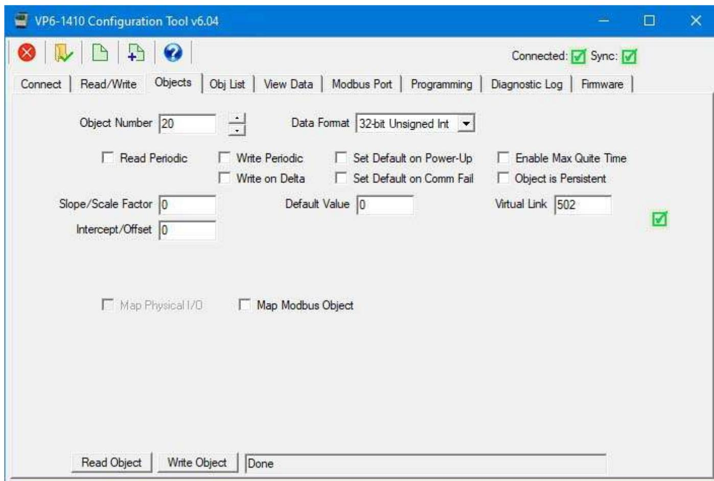
Example of usage: If you want to read via Modbus how many times the relay output DO 1 on the VP6-1410 (object 13) has turned on (cycle count), you would enter virtual link number 1013 in some otherwise unused object. Now read this object to see how many times the output has turned on.
