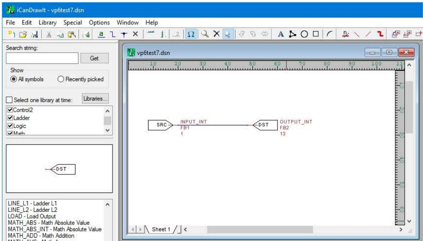
Click the green "i" icon next to the folder icon to open the i.CanDrawIt graphical programming tool that is illustrated below. It has its own set of help pages. Click on the "?" icon in that tool for more about programming. (Note that i.CanDrawIt is a second software package installed after the ValuPoint configuration tool - if you have trouble starting up i.CanDrawIt, be sure it was installed.)
