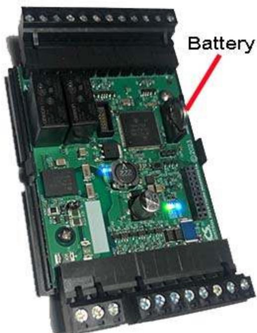
Replace battery with BR1225A only. Use of another battery may present a risk of fire or explosion. Replace with battery polarity as marked on the circuit board. Reverse polarity of the battery will not damage the board, but the clock will not be backed up if the battery is reversed.
