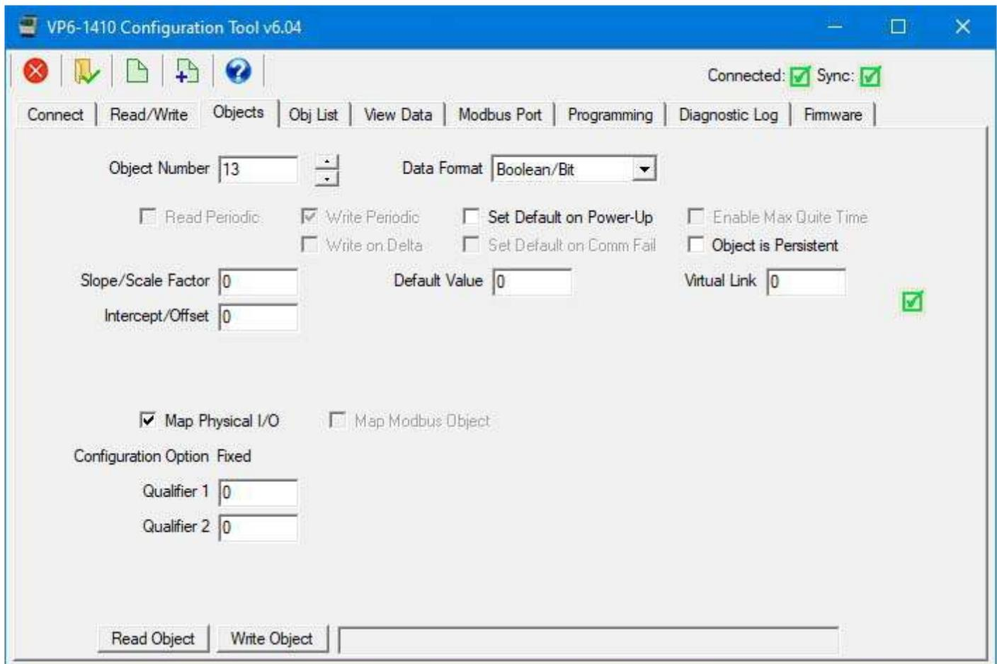
The above example illustrates the configuration for one of the relay outputs. There is really nothing to configure unless you want to do some special things like link the output to an input as illustrated later in this section.
