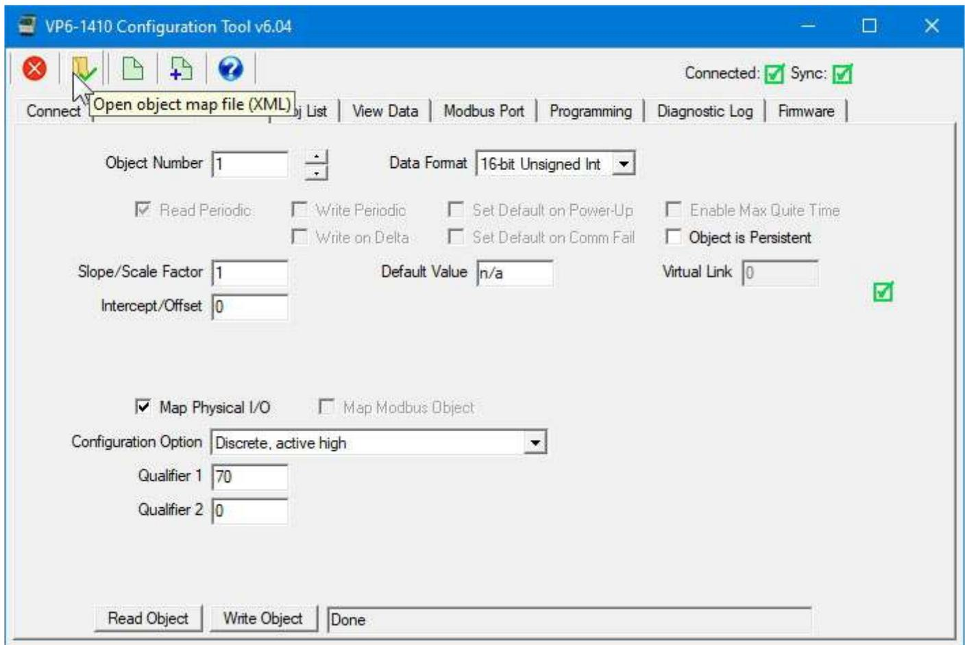
Click the "Save copy" icon to create a new XML file that contains all of the configuration settings currently displayed by the configuration tool. The icon just to the left will re-save an XML file that is already open.
