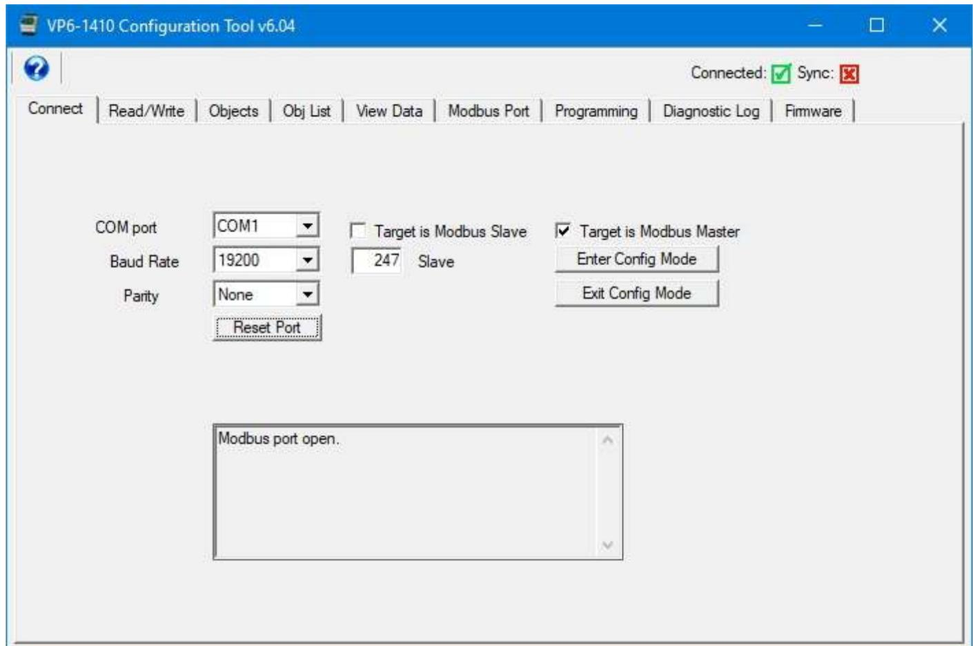
**IMPORTANT:** Do not change device mode to Modbus master until AFTER you have created some Modbus register mappings for the master to act upon. These are set up on the Objects page. If you switch to master mode without anything for the master to do, you will have trouble entering configuration mode. See Modbus Port page for more about this.
