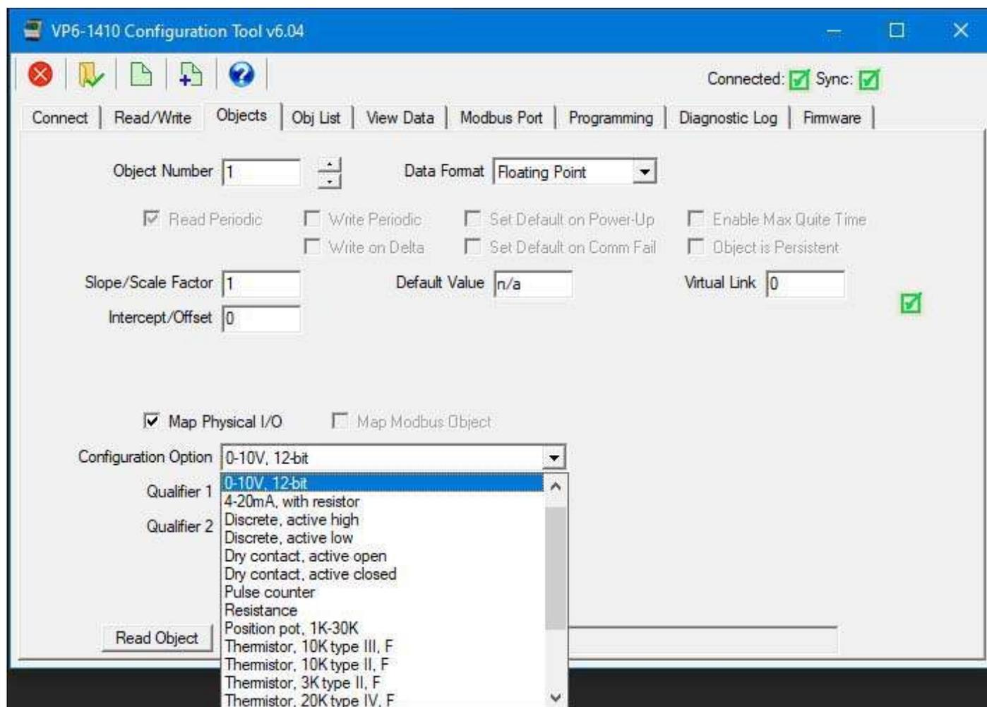
Objects 1-14 are permanently mapped to physical I/O points. While you cannot unmap them, you can change how the universal inputs are configured to operate.
