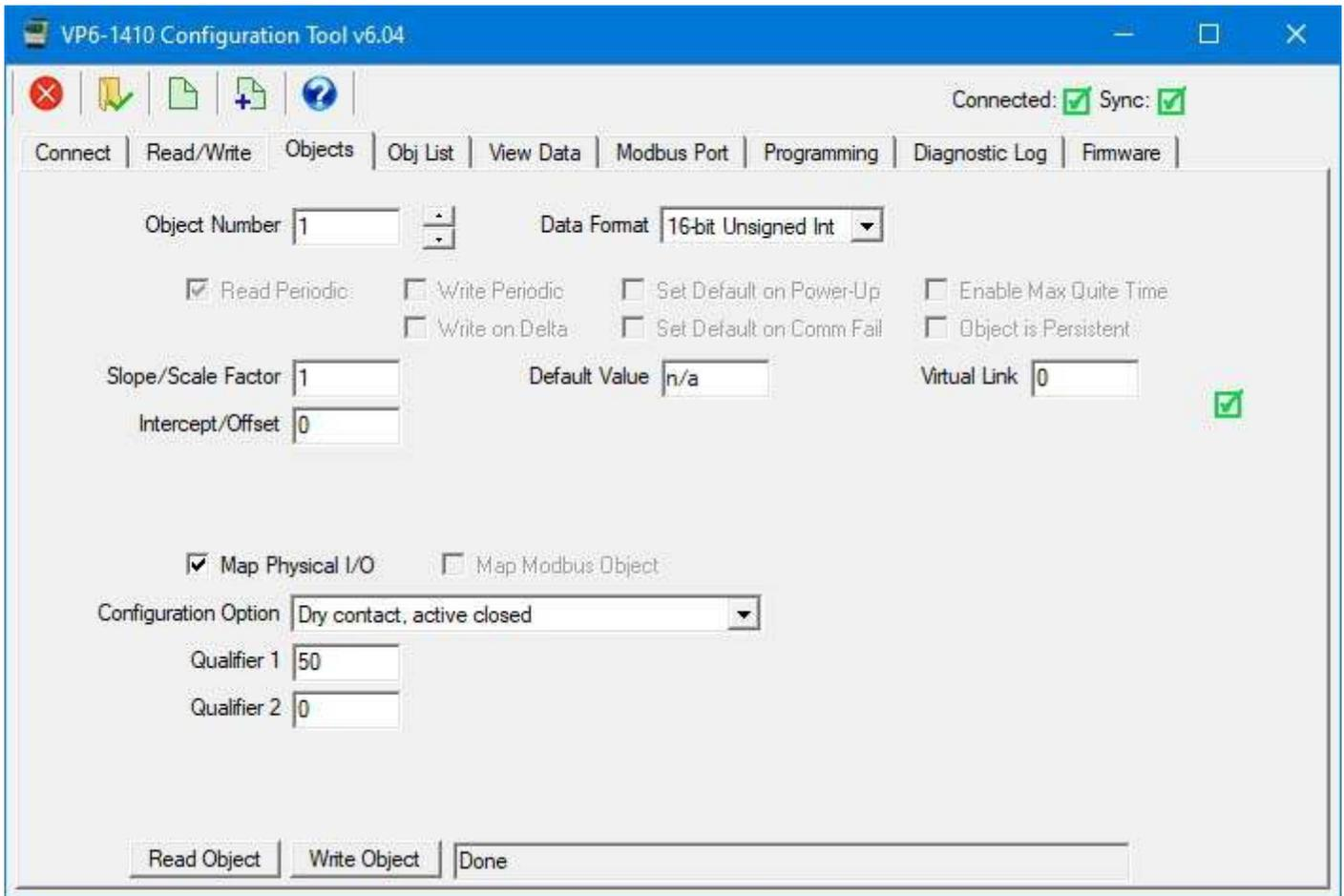
The programming environment only knows how to read/write 32-bit values. Therefore, select 32-bit integer as data format.
