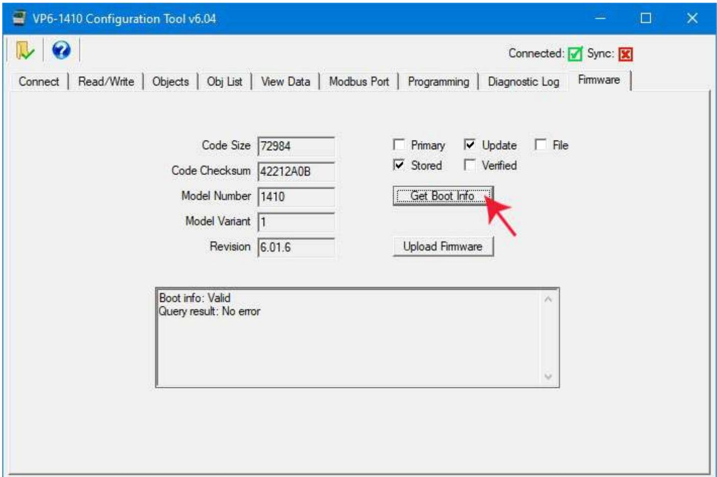
By selecting "Verified", you can cause the device to scan the code just uploaded and compare the checksum. You should get "Valid, No error" and this will indicate that the upload was successful and code has been verified.
