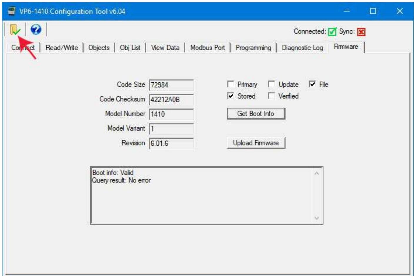
The upload process will take a couple of minutes. During this time, progress will continue to get posted to the status window. When the upload is complete, the boot info record for the update image is written.
