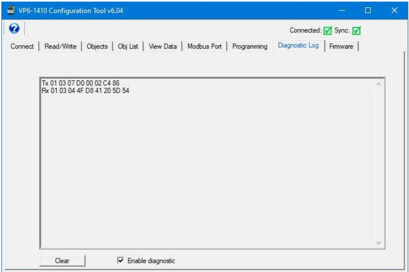
Note that only communication between the configuration tool and some other Modbus device are displayed here. Communication between two other Modbus devices will not be captured here. Only communication involving the tool is displayed.
