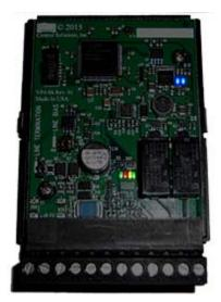
The LED indicators for the VP4-0610 are mounted on the circuit board inside the device, and are viewable through the vent slots in the case. The two blue LEDs are power indicators. There are two power supplies in the VP4-0610, and both are necessary for proper operation.
