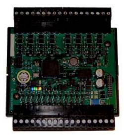
The LED indicators for the VP4-2810 are mounted on the circuit board inside the device, and are viewable through the vent slots in the case. The blue LED is the power indicator. There is one power supply in the VP4-2810.
