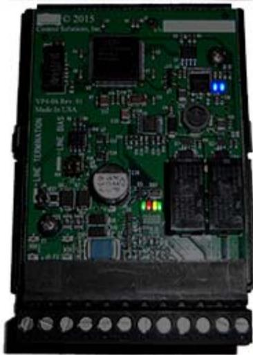
The LED indicators for the VP4-0630 are mounted on the circuit board inside the device, and are viewable through the vent slots in the case. The two blue LEDs are power indicators. There are two power supplies in the VP4-0630, and both are necessary for proper operation.
