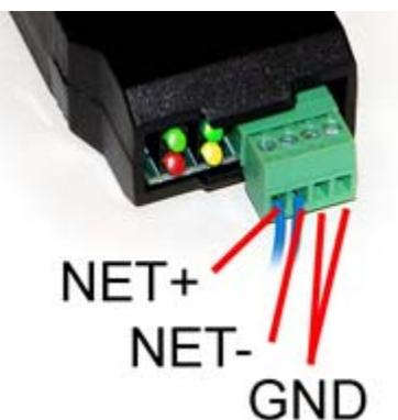
DO NOT connect power to the terminal block on the adapter. The adapter gets its power from the USB port of your PC. The adapter only draws a very small amount of power, well below the limit provided by standard USB ports.
