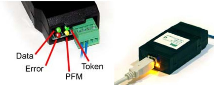
The yellow LED next to the USB connector will light up any time the PC recognizes this device. There is a blue power LED inside the adapter visible by looking into the adapter through the slot next to the USB adapter. The power LED should always be on if connected to the PC. The yellow LED will only come on when recognized by PC software.
