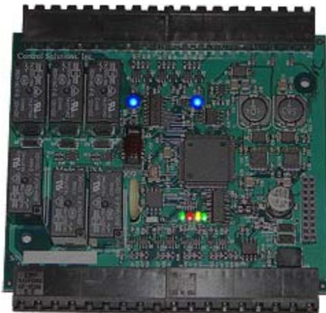
The LED indicators for the VP4-2330 are mounted on the circuit board inside the device, and are viewable through the vent slots in the case. The two blue LEDs are power indicators. There are two power supplies in the VP4-2330, and both are necessary for proper operation.
