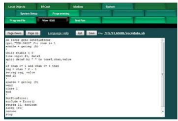
Script Basic can program your MX-71-SP to be a passive listener capturing data from something like a data logger. Script Basic can also program your MX-71-SP to be an active polling device to query your serial device and interpret the response to provide data to BACnet (or Modbus TCP).
