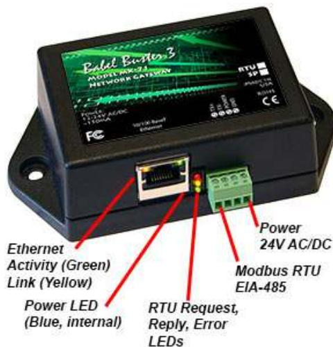
(b) Connect a CAT5 cable between the RJ-45 jack on the gateway, and your network switch or hub. You cannot connect directly to your PC unless you use a "crossover" cable (or your PC supports auto-MDX, which many newer laptops do).
