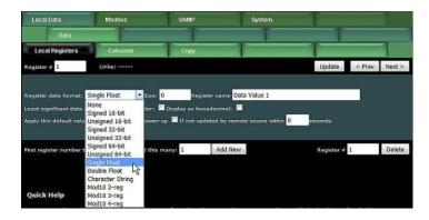
Configuration of the gateway is done via the secure web pages served by the internal web server. The user simply fills in templates. The entire configuration is saved in the internal Flash file system in XML format. This file may be exported to replicate additional copies of the configured device, or for backup.
