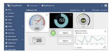
The MQ-73 also supports interactive dashboards using ThingsBoard. The MQ-73 includes features specific to ThingsBoard that allow MQTT interaction with graphic widgets on the dashboard. BACnet data published by the MQ-73 can show up as real-time gauge indications or charts. Input from the dashboard such as knob adjustments or switch changes will be immediately reported to the MQ-73 and those changes are immediately accessible as BACnet data.
