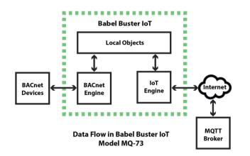
The data flow in the MQ-73 is illustrated above. Data is collected from BACnet devices by the BACnet engine which stores that data in local objects. The BACnet data is automatically updated on a continual basis. Meanwhile, the IoT engine is looking at its set of publish and subscribe rules to decide when to publish data from the local objects to the AWS server. These rules are also created by the user and data will be published according to the criteria set up by the user.
