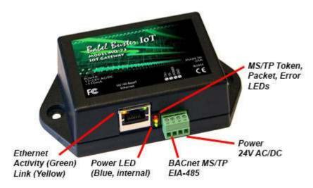
Babel Buster MQ-73 Token, Packet and Error LEDs reflect BACnet MS/TP traffic, and the Ethernet activity LED will indicate network traffic in general.
