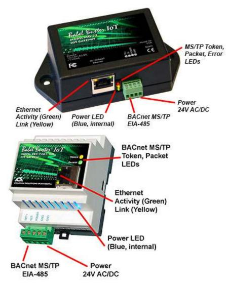
(b) Connect a CAT5 cable between the RJ-45 jack on the gateway, and your network
