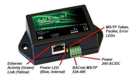
(a) Does the device have power? A blue LED inside the case, visible through the air vent slots, will be on if there is power present.
