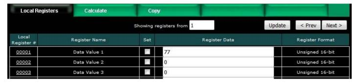
It is common for Modbus devices to pack a number of status bits into a single holding register. In order to do meaningful things based on a single bit, it is sometimes necessary to split that register into multiple local registers. Babel Buster supports this requirement by providing an optional bit mask.
