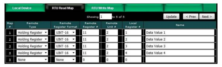
To try out these read maps, we have set up ModSim with the remote register 11 containing a value of 7.
