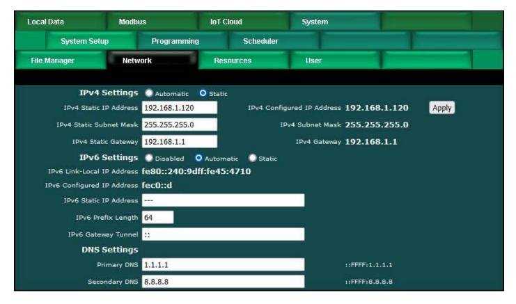
Most changes are stored in an XML configuration file in the device's Flash file system. Only a few are stored differently, and the IP address is one of those. Normally, clicking Update on any configuration page only stores that configuration information to a temporary RAM copy of the configuration file. To make your changes other than IP address permanent, you must execute Save XML Config File on the File Manager page (System :: System Setup :: File Manager). Refer also to section 3.1.
