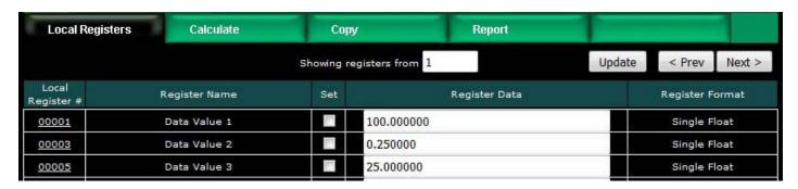
Constants may be introduced into the calculation by reserving a register to hold that constant, and then configuring it to apply a default value at power-up. This default value should be the constant you wish to include in a calculation.
