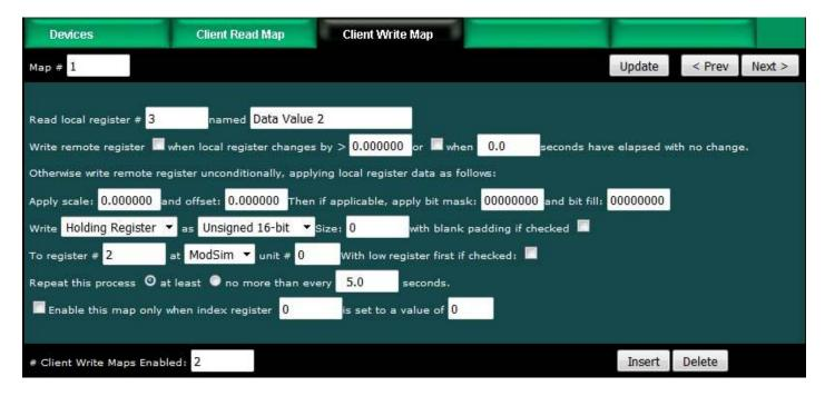
The local register data may be written to the remote device periodically, or when it changes, or both. To send upon change (send on delta), check the first box and enter the amount by which the local register must change before being written to the remote device. To guarantee that the remote register will be written at least occasionally even if the data does not change, check the second box and enter some amount of time. This time period will be referred to as the "maximum quiet time".
