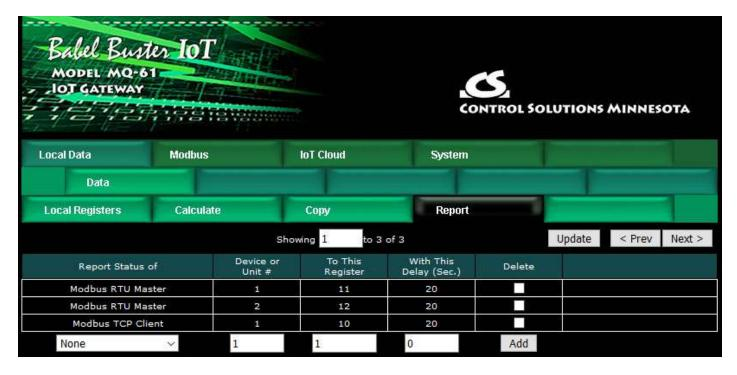
This optional list allows reporting device errors as register values to make it easier to monitor communication failures. The length of the list is variable. To add to the list, select the type of device to report on, select the device instance or unit number to report on, and select a register in which to put the status indication. Enter a delay if desired, and then click Add.
