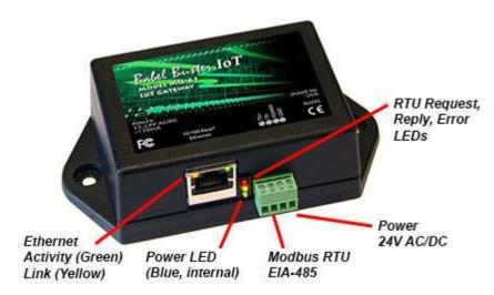
Babel Buster MQ-61 request/reply LEDs reflect RTU traffic while the Ethernet activity LED will indicate TCP traffic. To see TCP errors, one needs to look at the Errors page in the web UI.
