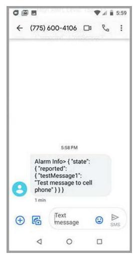
The combination of the Simple Notification Service set up in Section 16 and the simple test program illustrated here results in the text message being displayed on the mobile phone.
