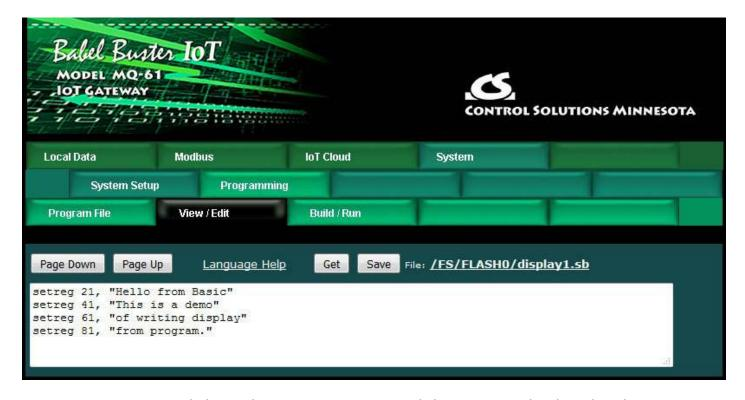
We are going to send this 4-line message to an alphanumeric display that has a Modbus RTU interface. To start out, we need to configure the Modus RTU port for the baud rate that matches the display. The Babel Buster will be the master since the display is an RTU slave.
