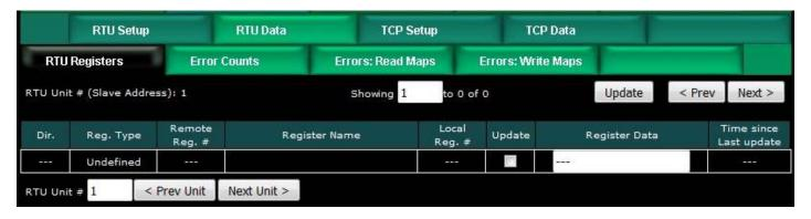
Click the Next Unit button to go to the next RTU slave, or simply enter a number in the RTU Unit # window and click Update. Registers for that slave will now be displayed. In addition to a summary of the map (both read and write maps are shown), the time since last update is displayed. This time should generally be less than the poll time. If the last update time is large, it means there is an error preventing the update.
