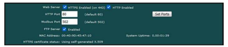
If there is a need to delete the self-generated certificates, you can do so by logging in via FTP. Change directory to /FLASH0, then to .cfg. The two certificate files that were self-generated are ssl.cert and ssl.key.
