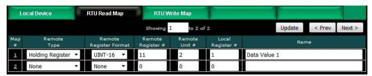
Enter the register number to read from the remote RTU slave and slave address of that RTU slave. Do not use Modicon numbers here. In other words, if your slave device's documentation says read register 40001, that is short hand (Modicon
