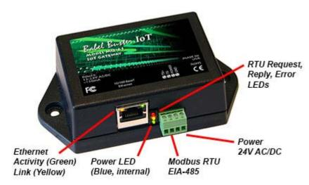
(b) Connect a CAT5 cable between the RJ-45 jack on the gateway, and your network switch or hub. You cannot connect directly to your PC unless you use a "crossover" cable.
