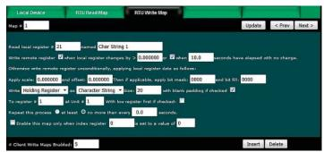
Interface to a Modbus RTU alphanumeric display device has never been easier. The Pro-V210 recognizes a series of Modbus holding registers as a single character string. The built-in Script Basic includes richly featured character string manipulation and recognizes the series of registers as a single character string.
