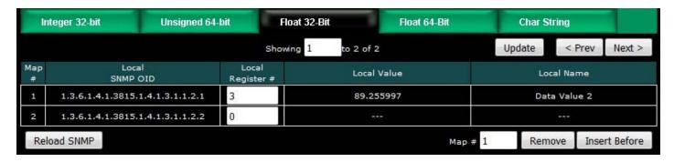
Local registers added to the Float 32-Bit MIB branch will be provided in IEEE 754 format per RFC 6340.
