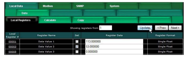
To test Setting the mapped OID, you can go to the Local Registers page, enter a new value for the local register, check Set, and then click Update. If monitoring traffic in Wireshark, you should see the request go out.
