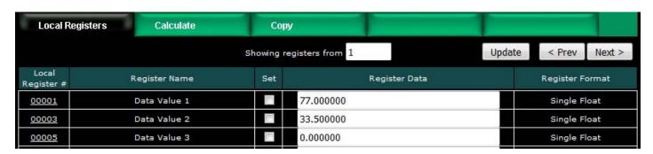
If the local register and remote register are not the same format, then data is converted automatically when written. In the example above, the Write Map is writing
