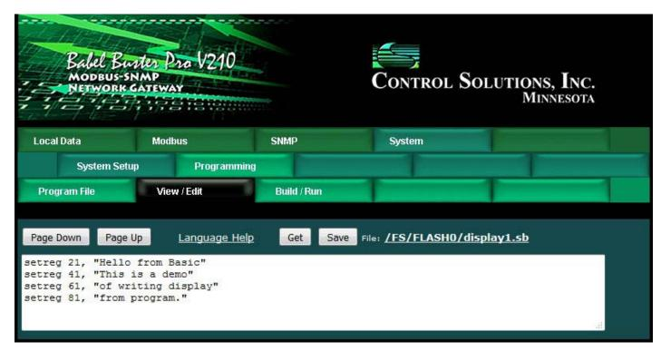
We are going to send this 4-line message to an alphanumeric display that has a Modbus RTU interface. To start out, we need to configure the Modus RTU port for the baud rate that matches the display. The Babel Buster Pro will be the master since the display is an RTU slave.
