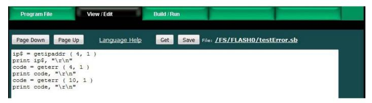
Normal results will be to display the IP address and two error codes that will be zero if there are no problems.
