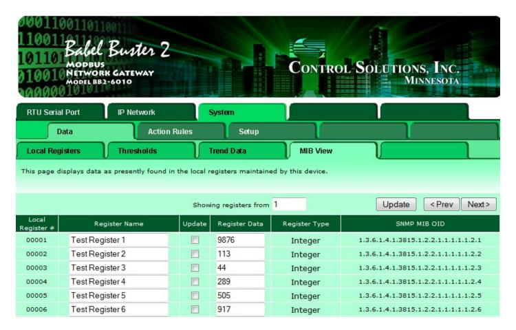
The screen shot of the walk rule list shows the previous example plus this example added as a second rule. Because this is a simple "Normal" table walk, everything needed can be entered on the tabular rule list. The first OID to be read is given as the table name. Select the device, starting local register and count, and poll rate. That is all that is needed. (Note: The device in this example has already been set up over on the devices page, first tab.)
