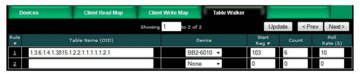
To select any table walk method other than Normal, you need to click on the table walk rule number in the first column, and select the method on the expanded view of the walk rule.
