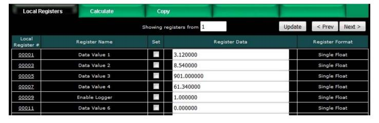
Once you have data appearing in the local registers, you can read them via Modbus TCP (or use the Modbus TCP client to write them to another Modbus TCP device). You do not need to configure anything in the local MIB in order to use Modbus TCP.
