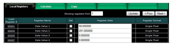
Upon restoring utility power, Data Value 1 returns to zero indicating we are no longer on battery power. Data Value 2 will continue to contain the last received "minutes remaining" value.
