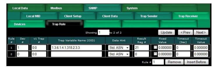
Rules for recognizing received traps are defined on this page. You have the option, on the System Setup Network page, to declare that trap receiving is disabled, or if enabled, processed by these rules and/or Script Basic programming.
