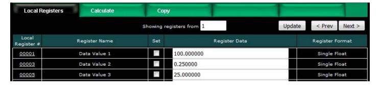
Constants may be introduced into the calculation by reserving a register to hold that constant, and then configuring it to apply a default value at power-up. This default value should be the constant you wish to include in a calculation.
