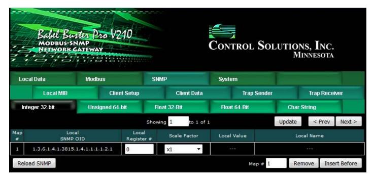
To add a local register to a MIB branch, simply enter the local register number at the next available OID which will always automatically be at the bottom of the list. When placing registers in the Integer branch, you also have the option of applying a scale factor. Scaled integer is the most universally recognized means of transmitting non-integer data.
