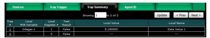
The thresohld has been exceeded in the above rule, and therefore a trap has just been sent in the illustration below.
