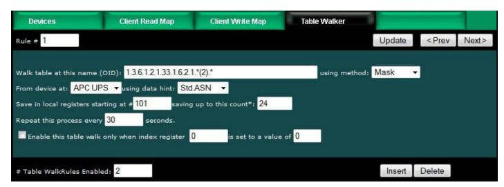
The resulting "UPS on battery" alarm, being alarm #2, sets bit 1 in the packed bit register 101 in our example. Alarm #1 sets the least significant bit, alarm #2 the next bit, and so on.
