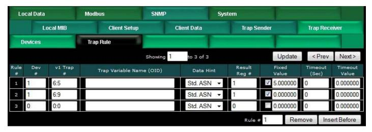
The resulting local register when utility power to the UPS is cut off in this example appears as follows:
