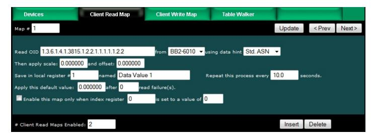
The optional scale and offset may be used if the value being read is scaled, or you may simply use scale and offset to perform units conversions. If non-zero, the received data will be multiplied by scale, then added to offset, before being placed in the local register.
