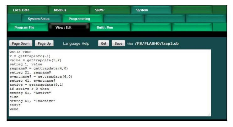
Whether writing a program or creating trap rules to receive a trap, you will need to know what you expect to find in the trap. This will be available in the MIB associated with the SNMP device you are receiving the traps from. You need to obtain this from the manufacturer of the SNMP device. In our example, the SNMP device is a Control Solutions BB2-6010, and the trap portion of its MIB is illustrated here.
