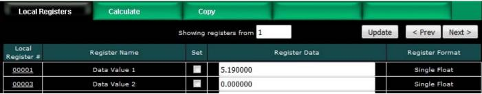
In this example, we have selected a scale factor fo x100. That means that our local value of 5.19 will be transmitted (in a Get response) as integer 519 and it is up to the recipient to know that this is scaled x100.
