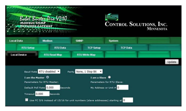
Select baud rate and parity from the drop down list. Click either Master or Slave buttons to select type of operation. Enter timing parameters or address as applicable. Click update to register your changes.
