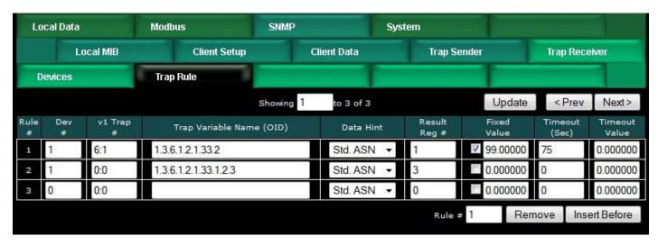
Immediately upon switching to battery power (utility power cut off), registers 1 and 2 are populated as illustrated below by the traps received from our test UPS. Data Value 1 is simply the fixed value flagging the fact that we are on battery power, and Data Value 2 is the number of minutes of remaining battery power provided by the UPS.
