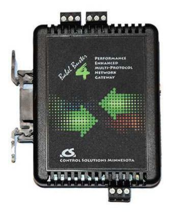
The BB4-8422 enclosure should look like the above photo when ready to DIN rail mount. Note that the "spring" in the clip is toward the bottom. To mount on the rail, hook the top of the clip in the rail, and push on the bottom of the enclosure until the bottom snaps in place on the rail.
