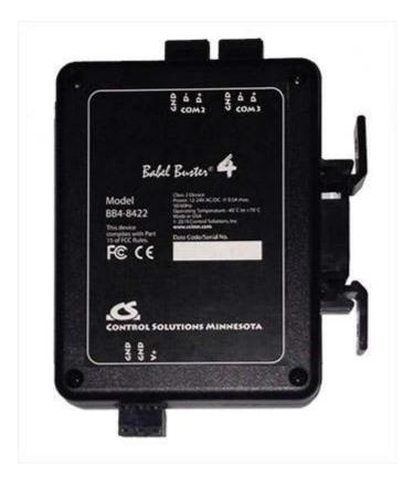
The connector pin-outs for the 3-position screw terminals are displayed on the back side of the BB4-8422. The D+ and D- are the positive and negative pins for RS-485 (EIA-485). These ports are electrically isolated from each other and from power.
