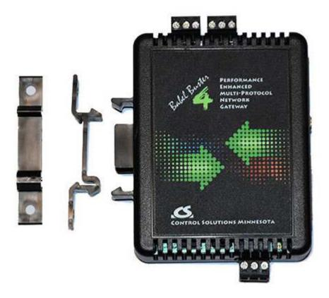
The BB4-8422 comes with a mounting bracket that can be used for either DIN rail mounting or wall mounting. To wall mount, start by screwing the bracket to the wall using the two screw holes in the bracket. Screws with washers are recommended (not included). To DIN rail mount, start by pressing the mounting bracket into the clips on the enclosure (this is normally the way the BB2-8422 will be shipped).
