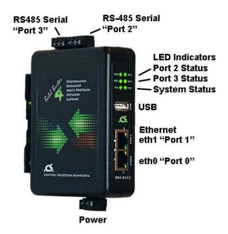
Port numbers are sometimes referred to generically just by number in the web UI in the BB4-8422. Ports 0 and 1 will always refer to Ethernet. Ports 2 and 3 will always refer to serial ports 2 and 3.
