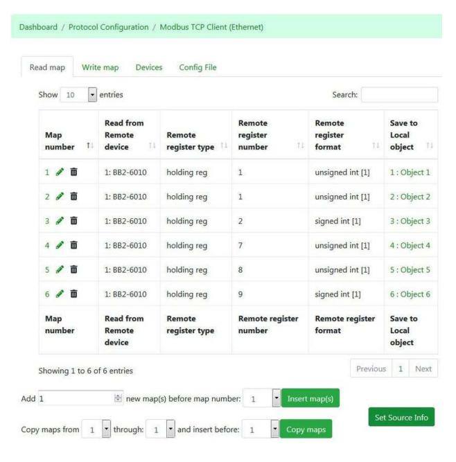
Modbus TCP Client Read Maps are where you configure this device to read Modbus registers from other Modbus TCP devices, and store that data in local data objects. This page shows a list of currently configured read maps.
