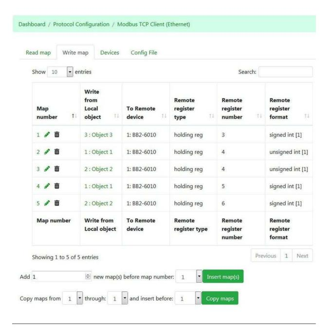
Modbus TCP Client Write Maps are where you configure this device to write to Modbus registers in other Modbus TCP devices, taking data to be written from local data objects. This page shows a list of currently configured write maps.
