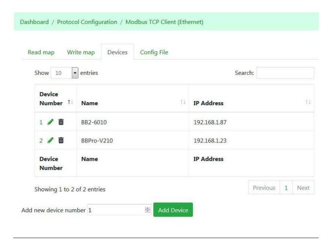
The Modbus TCP Devices page is where you set up the list of Modbus TCP servers (slaves) that this IoTServer will read from and write to while acting as a Modbus TCP client (master).
