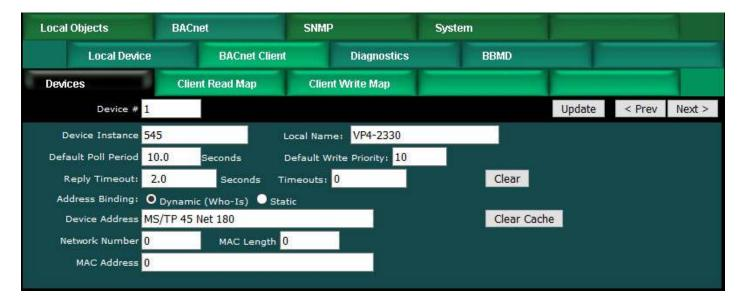
Much of the time, especially with BACnet IP, the client device timeout is the only timeout one needs to be pay much attention to. However, it is important to understand what is going on inside BACnet behind the scenes, especially if the client is making requests to an MS/TP device on the other side of a router.
