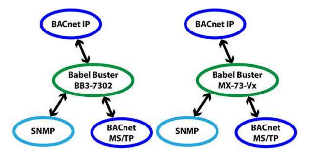
The most common application of the BB3-7302/MX-73 will be to use it simply as a BACnet Router. In this case, you do not need to concern yourself with any of the client read/write maps. These are not necessary for routing. You simply need to set up the network parameters, and communication between BACnet IP and BACnet MS/TP devices will happen automatically.
