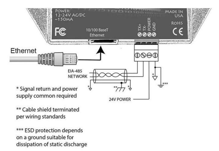
Wire the gateway as illustrated. Follow all conventional standards for wiring of EIA-485 networks when connecting the MS/TP EIA-485 (RS485) network. This includes use and termination of shield, termination of the network, and grounding.
