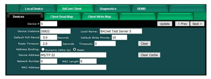
Include network number, mac length, and mac address ONLY if static binding to a device on the other side of some other BACnet router. In the example below, the device is an MS/TP device at MAC address 22 on network 115 on the other side of a router at 192.168.1.115 which is connected to the local IP network.
