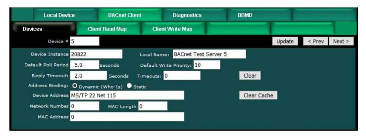
If static binding must be used, enter the fixed IP address you know the device instance to be found at. If no port is given, it will default to 0xBAC0 (47808). Enter IP as a.b.c.d or IP with port as a.b.c.d:p, for example 192.168.1.99:47808. Network number 0 means local IP network. If the device is on the other side of a router, the MAC Address entry must be used instead.
