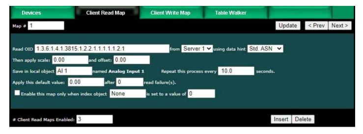
The optional scale and offset may be used if the value being read is scaled, or you may simply use scale and offset to perform units conversions. If non-zero, the received data will be multiplied by scale, then added to offset, before being placed in the local object.
