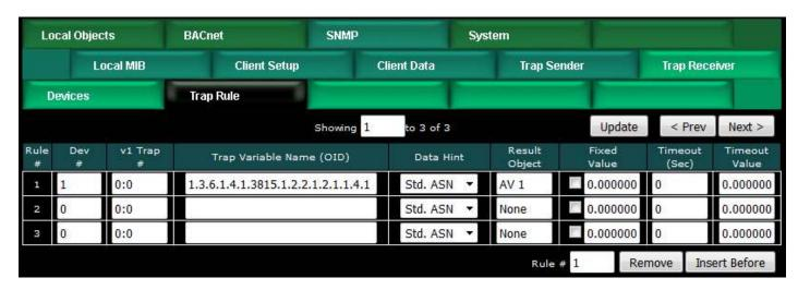
The Wireshark capture of a trap from this v2 device is illustrated below. In this case, the OID in the trap rule identifies a numeric (floating piont) value that is sent as an
