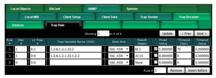
Now each trap will set Binary Input 1 to Active, and also place the minutes remaining in Analog Input 15.
