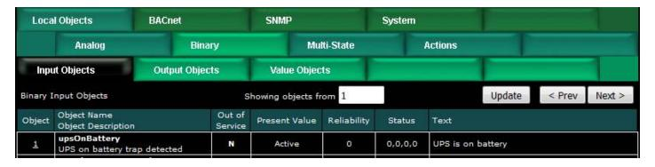
In addition to the trap number itself, the trap includes some varbinds (data pairs consisting of an OID and the data value identified by that OID). Rule #2 in the next example will capture the remaining minutes of battery power sent by the UPS with each of those trap messages sent every 60 seconds. Although this is still a v1 trap, it is important to leave the trap number set to 0:0 so that the varbind is processed by the rule rather than the trap number.
