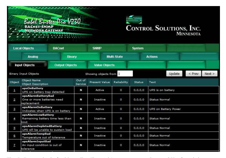
The Index method of table walk will set objects corresponding to OIDs found that reference the "well known alarms" defined in RFC 1628. Objects are skipped if no corresponding OID is found in the table. That means the Index walk will set objects but never clear them. To get the objects to reset after being set to indicate an alarm, the timeout feature of the table walk rule must be used.
