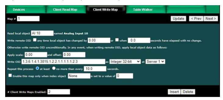
The local object data may be written to the remote SNMP device periodically, or when it changes, or both. To send upon change (send on delta), check the first box and enter the amount by which the local object must change before being written to the remote device. To guarantee that the remote OID will be written at least occasionally even if the data does not change, check the second box and enter some amount of
