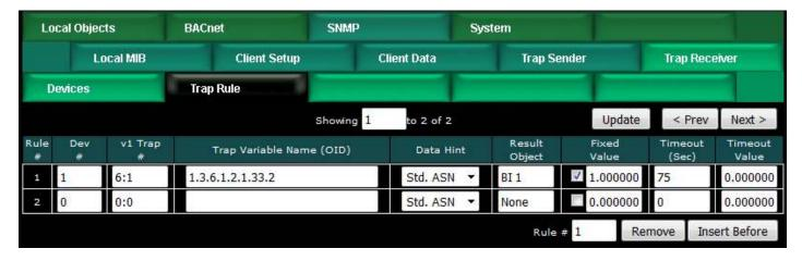
Rules for recognizing received traps are defined on this page. Rule number simply tells you where you're at on the list of Trap receiver rules. Click "next" and "prev" to scroll through the list. To advance directly to a specific rule, enter the desired number in the "Showing" box, then click Update.
