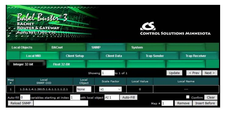
To add a local object to a MIB branch, simply enter the local object number at the next available OID which will always automatically be at the bottom of the list. When placing objects in the Integer branch, you also have the option of applying a scale factor. Scaled integer is the most universally recognized means of transmitting non-integer data.
