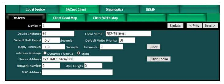
If the device is on the local MS/TP link then enter its MS/TP MAC address as the device address using "MS/TP" followed by the address. Network number 0 means local MS/TP network. If the device is on the other side of a router, the MAC Address entry must be used instead.
