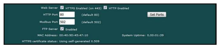
If there is a need to delete the self-generated certificates, you can do so by logging in via FTP. Change directory to /FLASH0, then to .cfg. The two certificate files that were self-generated are ssl.cert and ssl.key.
