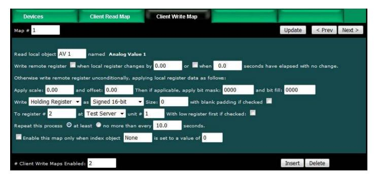
The local object data may be written to the remote device periodically, or when it changes, or both. To send upon change (send on delta), check the first box and enter the amount by which the local object must change before being written to the remote device. To guarantee that the remote register will be written at least occasionally even if the data does not change, check the second box and enter some amount of time. This time period will be referred to as the "maximum quiet time".
