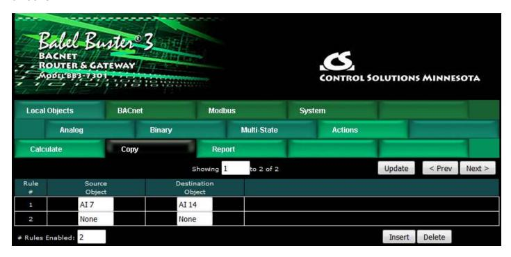
The above rule would cause the value of AI 7 to be placed in AI 14. If a floating point (Analog) value is copied to a Binary object, the Binary object will be set Active if the value was nonzero, or cleared to Inactive if zero. Analog values copied to a Multistate object will be not only truncated, but bounded to the maximum number of states (not a recommended use of Copy).
