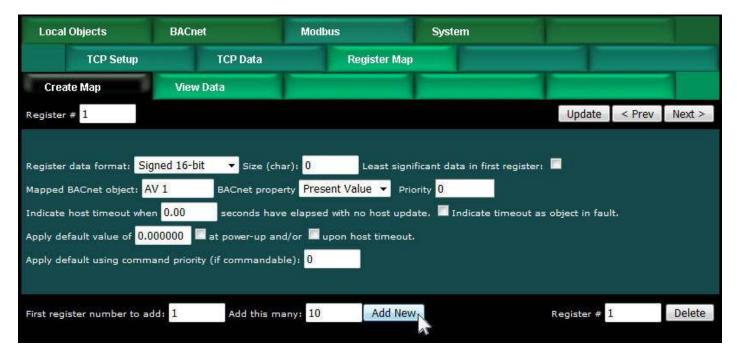
Upon clicking Add New with the above screen showing, we will create 10 Modbus registers assigned one each to a series of Analog Value objects as illustrated below. Return to this tabular view by clicking the Create Map tab again.
