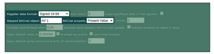
The BACnet objects are designated by a 2-character abbreviation followed by an object number. The object abbreviations are as shown below. The object must exist within the Babel Buster before it is allowed to be referenced here.
