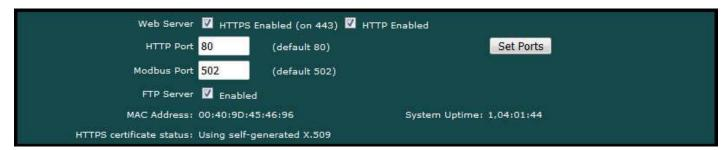
Secure browsing can be enabled here, and non-secure can be disabled. You cannot disable both, and a forced configuration reset will restore HTTP (non-secure) web browsing. In order to use HTTPS, you must first upload the necessary SSL certificates
