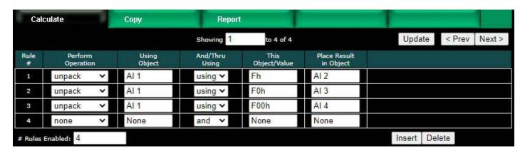
The pack, fill, and unpack instructions are primarily targeting Modbus applications.
