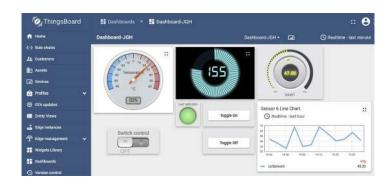
The BB3-7301-MQ also supports interactive dashboards using Things-Board. The BB3-7301-MQ includes features specific to ThingsBoard that allow MQTT interaction with graphic widgets on the dashboard. BACnet data published by the BB3-7301-MQ can show up as real-time gauge indications or charts. Input from the dashboard such as knob adjustments or switch changes will be immediately reported to the BB3-7301-MQ and those changes are immediately accessible as BACnet data.
