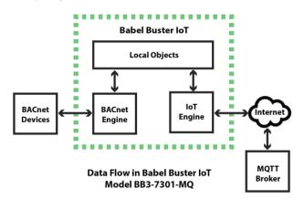
The data flow in the BB3-7301-MQ is illustrated above. Data is collected from BACnet devices by the BACnet engine which stores that data in local objects. The BACnet data is automatically updated on a continual basis. Meanwhile, the IoT engine is looking at its set of publish and subscribe rules to decide when to publish data from the local objects to the AWS server. These rules are also created by the user and data will be published according to the criteria set up by the user.
