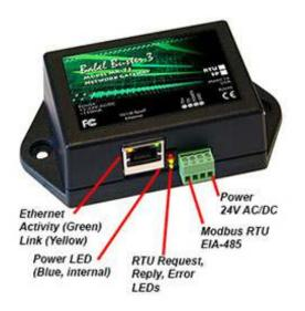
Babel Buster MX-71 Request, Reply and Error LEDs reflect Modbus RTU traffic, and the Ethernet activity LED will indicate network traffic in general.
