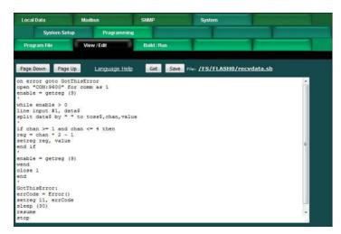
Script Basic can program your BB3-6101 to be a passive listener capturing data from something like a data logger. Script Basic can also program your BB3-6101 to be an active polling device to query your serial device and interpret the response to provide data to SNMP (or Modbus TCP).
