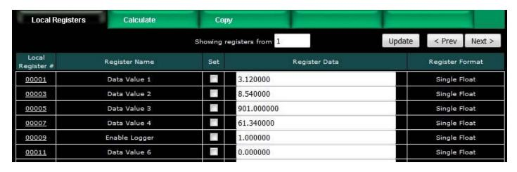
We are going to make these data values available via our own internal MIB so that other SNMP devices can do an SNMP Get to retrieve these numbers. To do this, we configure the local MIB to reference the registers we are using. Note that while our
