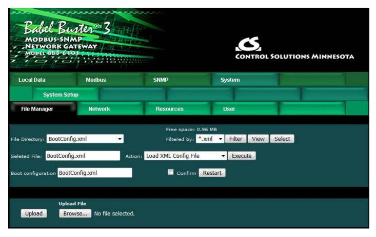
The File Directory is a list of files that are currently stored in the Babel Buster's Flash file system. To filter files by type, select a type from the Filtered by list, and click Filter.
