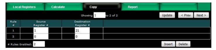
The above rule would cause the following copy to happen. Note that "copy" also means data reformatting. Therefore, if you need to convert a number to a character string (or vice versa), simply copy it from one register to the other. In this example, our copy rule is converting floating point to an ASCII string ready to be sent to a display device.
