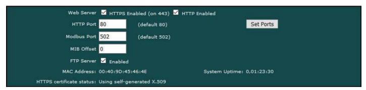
If there is a need to delete the self-generated certificates, you can do so by logging in via FTP. Change directory to /FLASH0, then to .cfg. The two certificate files that were self-generated are ssl.cert and ssl.key.
