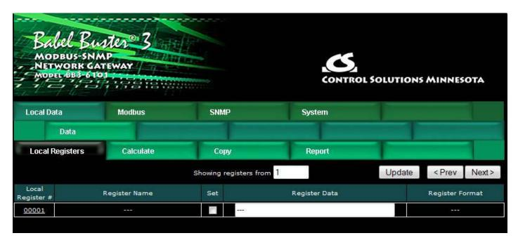
To begin the process of creating registers, click on the only register number available at this point. Later on, click on the register number at the end of the list to add more, or click anywhere in the middle of the list if there are gaps in the register number sequence that you would like to fill.
