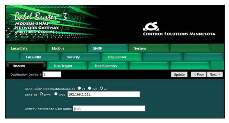
Traps may be sent as v1, v2c or v3. The same application varbinds will be included in either trap type, in addition to header and varbinds required for that trap type. (Note: We use the term "trap" generically here. The v2c/v3 "trap" is properly known as a Notification.)
