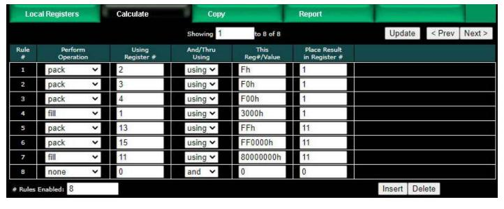
The example below shows the content of result registers 1 and 11 using the above calculate rules and the local register values shown. The contents of registers 2, 3, and 4 are packed into register 1. The contents of registers 13 and 15 are packed into 11 (all 32-bit register pairs).
