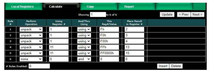
Register 1 is unpacked into registers 2, 3 and 4. Register 11 is unpacked into registers 13 and 15 (all 32-bit register pairs).
