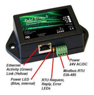
Babel Buster MX-61 Request, Reply and Error LEDs reflect Modbus RTU traffic, and the Ethernet activity LED will indicate network traffic in general.
