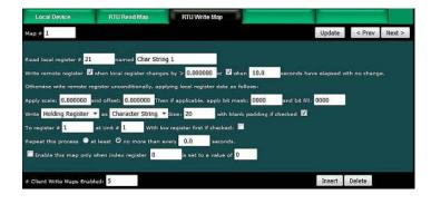
Interface to a Modbus RTU alphanumeric display device has never been easier. The BB3-6101 recognizes a series of Modbus holding registers as a single character string.
