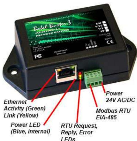
Babel Buster MX-61 Request, Reply and Error LEDs reflect Modbus RTU traffic, and the Ethernet activity LED will indicate network traffic in general.
