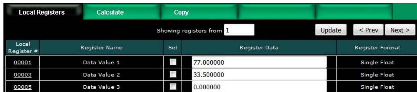
The screenshot shows a software interface for configuring Modbus registers. At the top, there are buttons for "Local Registers", "Calculate", and "Copy". Below these, a status bar indicates "Showing registers from 1" with "Update", "< Prev", and "Next >" buttons. The main part of the interface is a table with the following columns: "Local Register #", "Register Name", "Set", "Register Data", and "Register Format".
