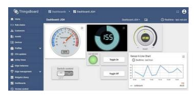
The BB3-6101-MQ also supports interactive dashboards using Things-Board. The BB3-6101-MQ includes features specific to ThingsBoard that allow MQTT interaction with graphic widgets on the dashboard. Modbus data published by the BB3-6101-MQ can show up as real-time gauge indications or charts. Input from the dashboard such as knob adjustments or switch changes will be immediately reported to the BB3-6101-MQ and those changes are immediately accessible as Modbus data.
