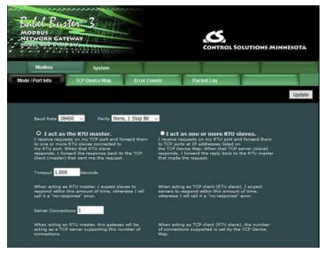
Accessing one or more Modbus RTU slaves from TCP with the external Modbus TCP device acting as client (master) means the gateway needs to act as an RTU master on the RTU network. Select "I act as the RTU master" for mode. You do not need to do anything on the TCP Device Map page for this mode.
