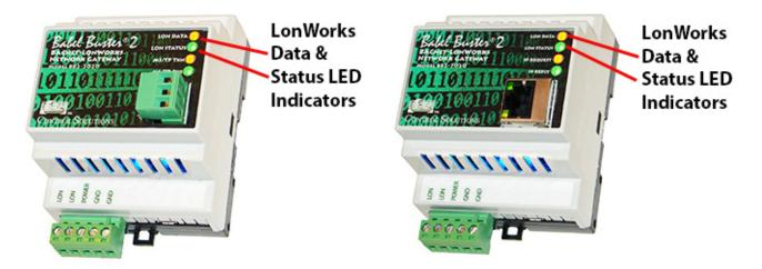
The LonWorks indicator LEDs display LonWorks network activity. Note, however, that activity of these LEDs is not only affected by configuration of the device, but by whether the device is commissioned on the network and whether other devices are also communicating.
