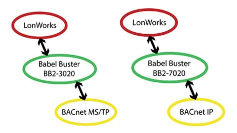
Babel Buster model BB2-3020 is a LonWorks to BACnet MS/TP gateway. It has two processors, an ARM7 and an Echelon FT5000. The FT5000 is running the LonWorks Short Stack microserver, and acts as a LonWorks communications port for the main application running on the ARM7.
