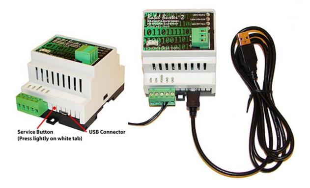
Use your PC's device manager (found in the control panel) to locate the COM port that the gateway appears on once connected via USB. Select this COM port on the Connect page of the tool, and click Connect.
