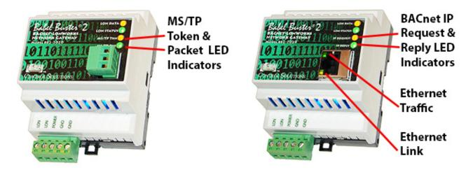
The MS/TP or IP LEDs will indicate BACnet traffic as indicated in the tables below.
