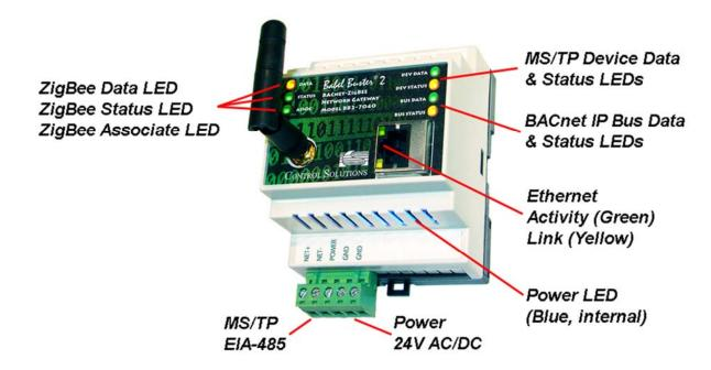
Upon power-up, the embedded server will take about a minute to boot up. A blue LED should be visible inside the device indicating power is present. Both the Ethernet Link and Activity LEDs should light up upon power-up assuming Ethernet is connected to a switch. After bootup, the Link LED indicates a network connection is present, and the Activity LED will flash any time network traffic is detected.
