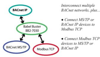
Provides Connectivity Between BACnet IP and MS/TP and Modbus TCP or SNMP
