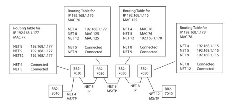
Router configuration required for test scenario of BB2-3010 gateway reading an Analog Input from BB2-7040 via a string of four routers alternating between IP and MS/TP.
