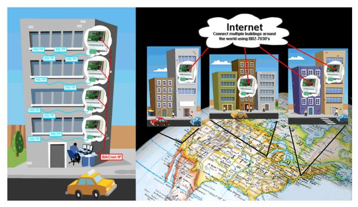
The BB2-7030 includes proxy support such that devices that do not support dynamic binding (Who-Is, I-Am) can be represented by proxy by the BB2-7030. The BB2-7030 will act as proxy for both MS/TP and BACnet IP devices.
