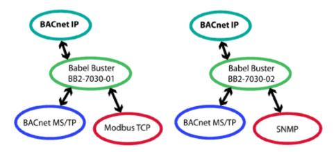
The BB2-7030-01 may be used as a gateway to connect BACnet MS/TP or BACnet IP to Modbus TCP. The connection of BACnet IP to Modbus TCP is also accomplished by the BB2-7010-01, but only the BB2-7030-01 can connect BACnet MS/TP to Modbus TCP.
