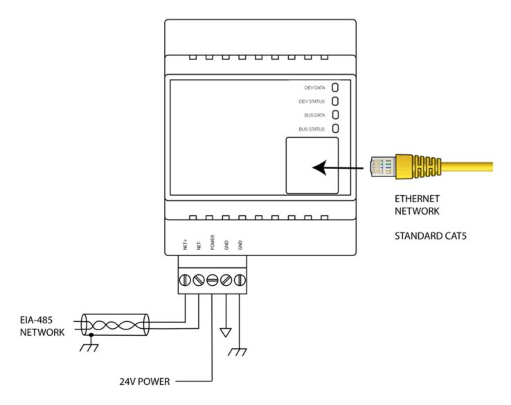
Wire the BB2-7030 as illustrated above. Follow all conventional standards for wiring of EIA-485 networks when connecting the MS/TP EIA-485 (RS485) network. This includes use and termination of shield, termination of the network, and grounding.
