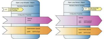
The LonWorks Network Variables (NV's) contained within the Babel Buster gateway are configured as standard sensor and actuator function blocks with user changeable network variable types. Each variable has been allocated the maximum of 31 bytes of memory, meaning any known LonWorks variable type (including UNVTs) can be used. The NV's are bound to other nodes on the LonWorks network using LonMaker or other comparable network management tool.
