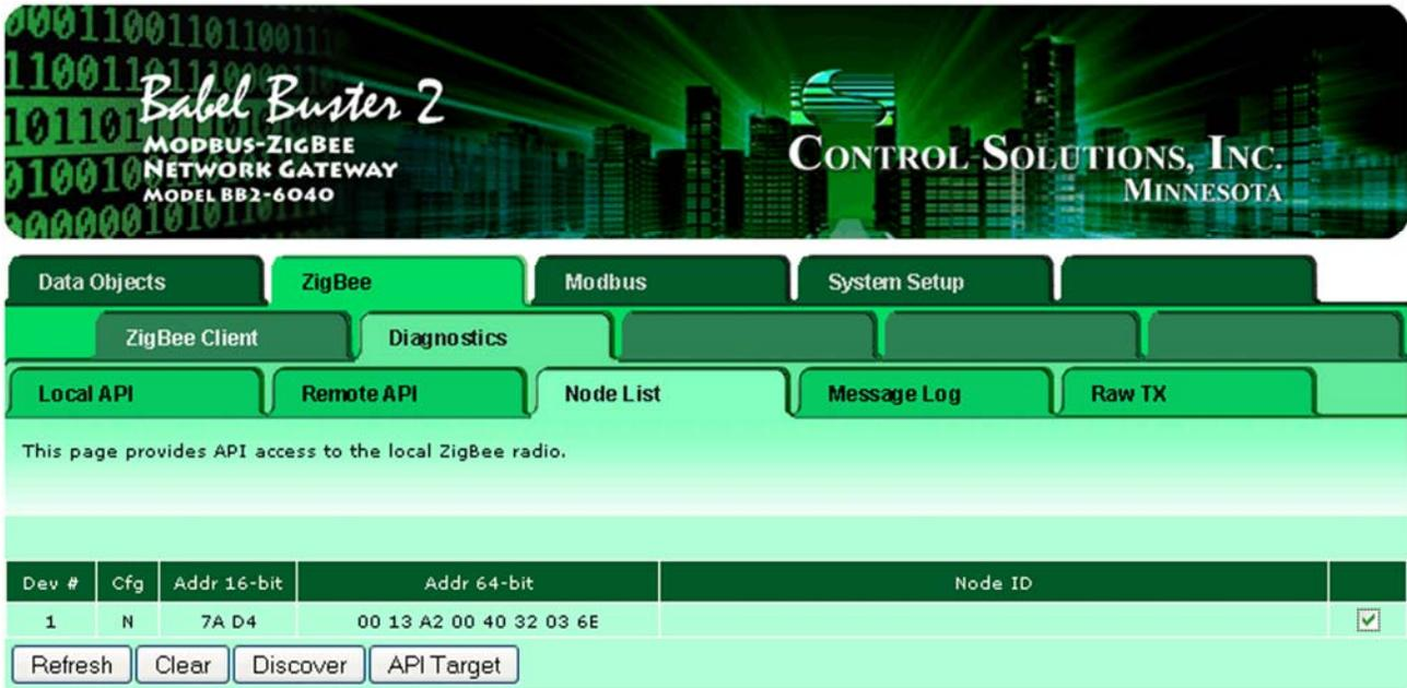
When a device is first connected, it will hopefully show up in the Node List. For this to happen, it must be configured with the same stack profile as the BB2-6040 (ZS parameter), and must be set for the same PAN ID, or set to “join any” PAN. Devices configured to use AT mode instead of API mode will also not show up here, but that does not mean you cannot communicate with them. Check the Message Log page to see if your device is sending anything the BB2-6040 can hear.
