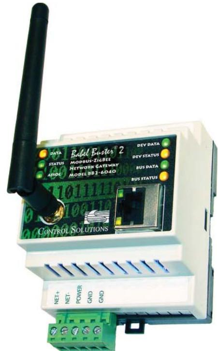
NOTE: If the yellow Link LED is not on, check your cable connections. It should be on any time power is applied and an Ethernet connection is present.
