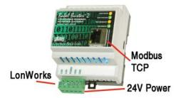
The BB2-6020-NB can poll up to 300 LonWorks network variables, each having up to 31 bytes of data. The BB2-6020-NB provides up to 400 Modbus registers which are used to exchange data with the LonWorks network variables.
