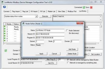
The Device Manager Configuration Tool is a user friendly LonWorks gateway configuration that runs on your PC. Connect the gateway to your laptop via a USB cable - no need for any adapters or "dongles", and no need to have a functional network on either side of the gateway for initial setup.
