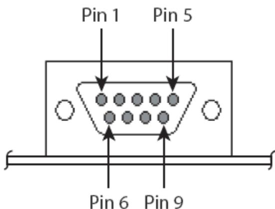
The above view is the male DB9 as seen looking into the Babel Buster SP. Important: This is **NOT** a PC COM port. Study the wiring table below carefully. Also keep in mind that while Pin 1 is on the left on the male connector, Pin 1 will be on the right looking at the female connector.
