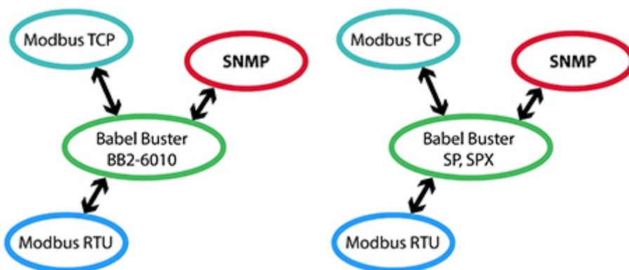
The most common application for these gateways is interfacing a Modbus device to an SNMP network, or vice versa. Another common application is remapping registers from multiple slave devices to appear as a single device on the alternate network, mapping RTU to TCP or vice versa.
