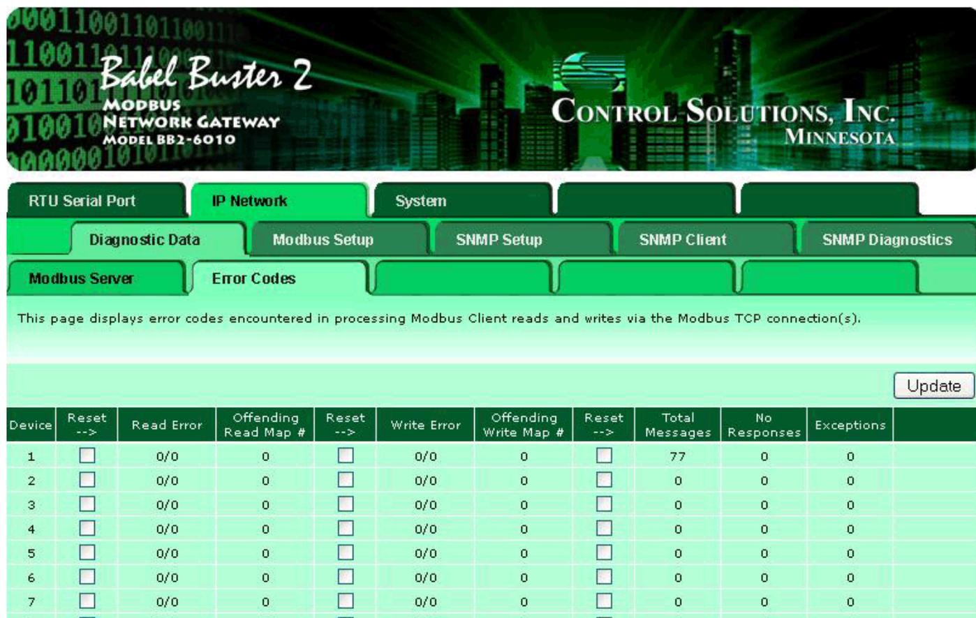
This page displays error codes encountered in processing Modbus Client reads and writes via the Modbus TCP connection(s).
