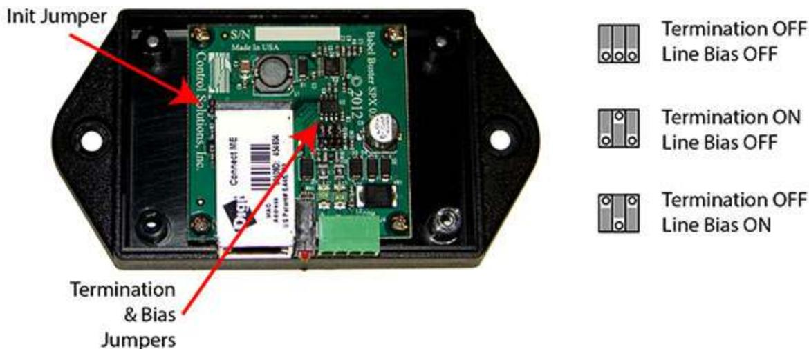
The "Init" jumper on the server module should only be used when advised by tech support. Installing this jumper prior to power-up causes the server to go into firmware update mode.
