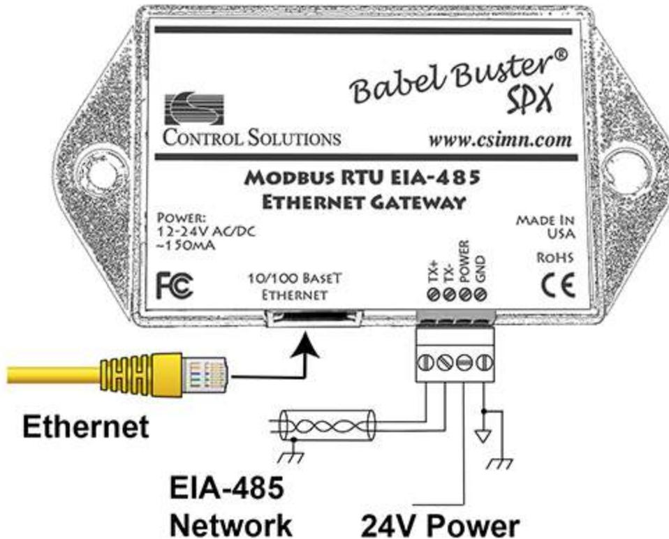
Wire the gateway as illustrated. Follow all conventional standards for wiring of EIA-485 networks when connecting the Modbus RTU EIA-485 (RS485) network. This includes use and termination of shield, termination of the network, and grounding.
