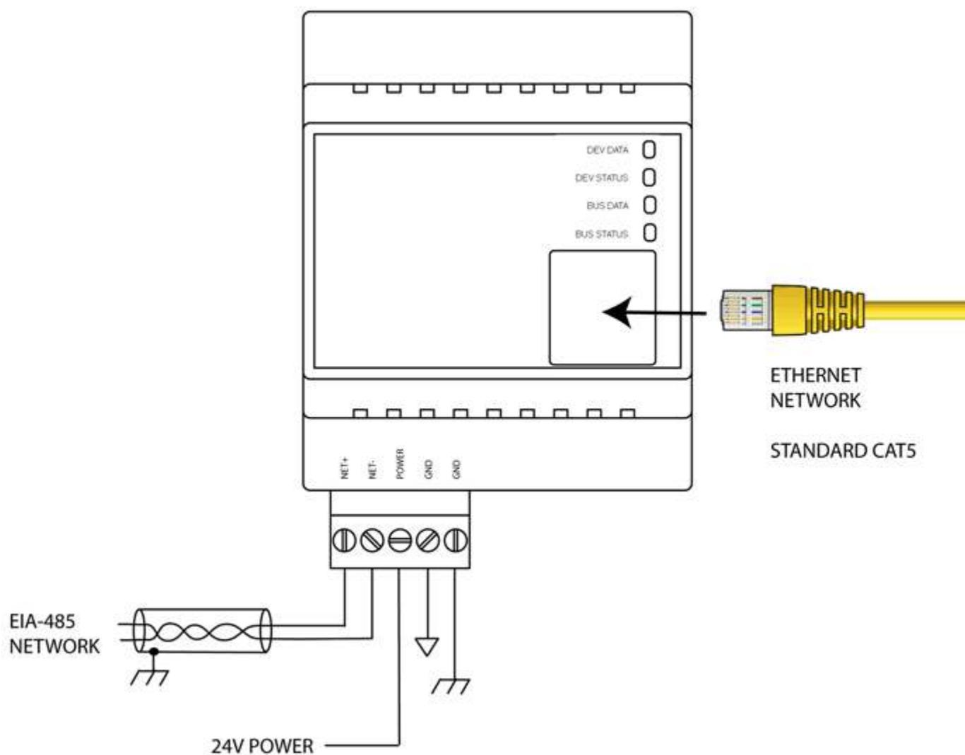
Wiring for the Babel Buster SPX is illustrated below (see section A.4 for SP).
