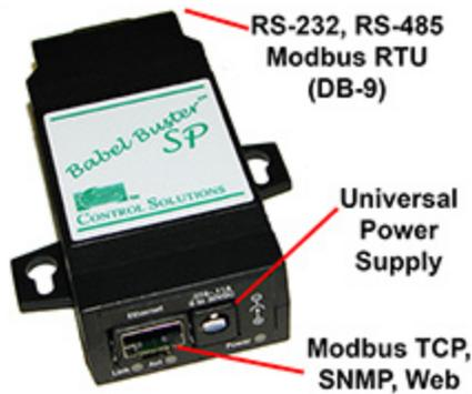
(b) Connect a CAT5 cable between the RJ-45 jack on the gateway, and your network switch or hub. You cannot connect directly to your PC unless you use a "crossover" cable.
