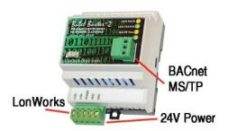
The BB2-3020-NB can poll up to 300 LonWorks network variables, each having up to 31 bytes of data. The BB2-3020-NB provides up to 300 BACnet objects which are used to exchange data with the LonWorks network variables.
