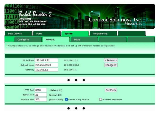
The abbreviated view of the Network setup page in an MQ-61 is illustrated below, and again the port has been changed to 8888 in this example.
