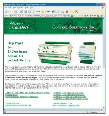
Online help included on the support CD or downloaded from our web site includes wiring diagrams, sensor calibration tool, BACnet object map, configuration tool user guide, and programming language help. Our source level program simulator and debugger is also free. Our PC based configuration tool simplifies setup of analog input type and scaling, and discrete I/O timing parameters.
