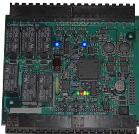
The LED indicators for the VP4-2310 are mounted on the circuit board inside the device, and are viewable through the vent slots in the case. The two blue LEDs are power indicators. There are two power supplies in the VP4-2310, and both are necessary for proper operation.
