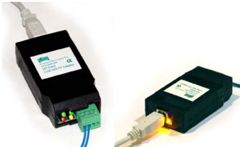
MTX002 USB to MS/TP Adapter
