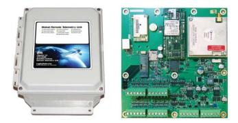
Control Solutions' i.Report Model VP4-2090 Global Remote Telemetry Unit is ideal for demanding remote alarm monitoring and data logging with optional GPS tracking. It includes both cellular and satellite radios built in. The model VP4-2090 can operate on cellular only, satellite only, or cellular with satellite backup for mobile applications. The optional GPS receiver provides tracking data for mobile applications.
