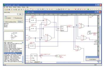
The i.Report Model VP3-3690 includes a field programmable soft PLC. Control Solutions' i.CanDrawIt® graphical programming tool is used to easily create programs.
