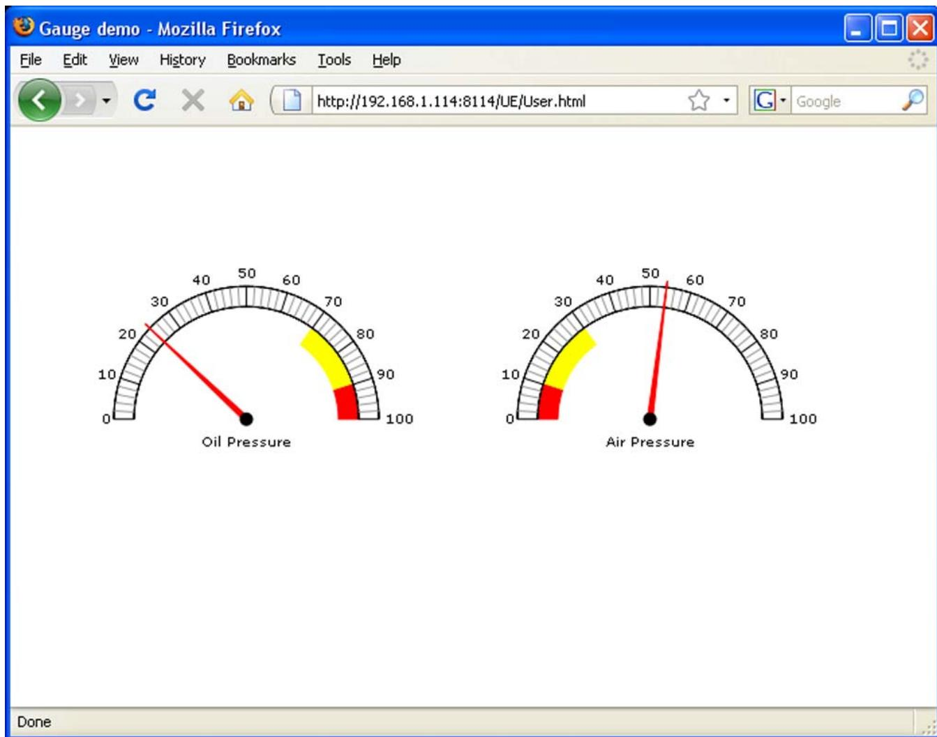
The needles on our gauges move in real time as data changes. In this case, data is being obtained from inputs on a AddMe Jr. The scale, labels, etc., may be changed and you may have any number of gauges on the page.
